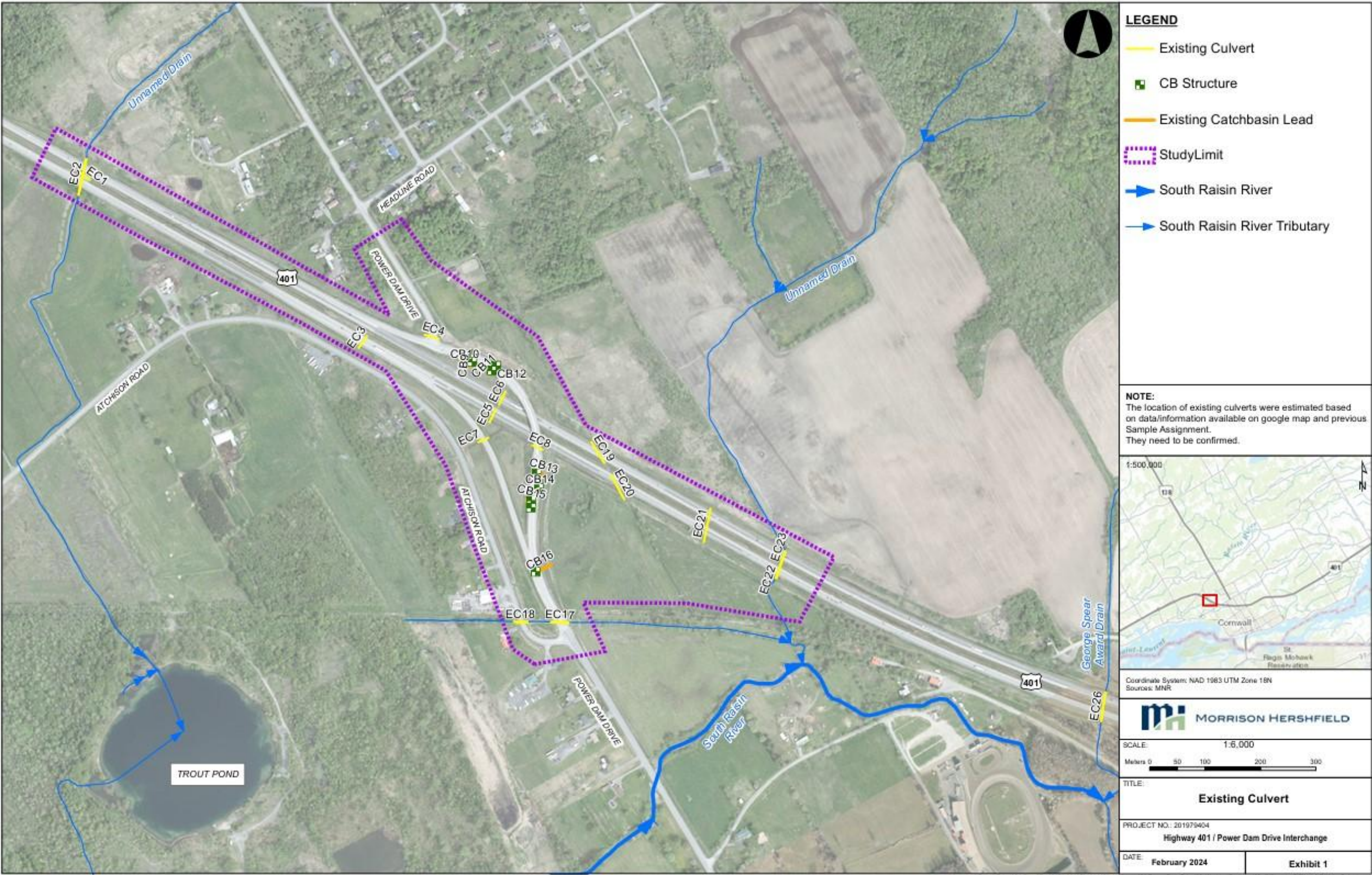
Figure 8: Existing Culverts Located within the Study Area
